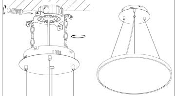
4. Push the canopy up towards the bracket, and rotate clockwise to secure. Tighten the 4 screws on the bracket to secure canopy. Installation is completed.
