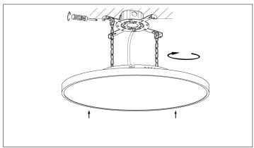
4. Push the canopy up towards the bracket, and rotate clockwise to secure. Tighten the 4 screws on the bracket to secure canopy.
