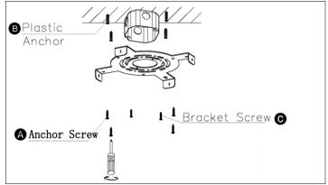
2. Install the mounting bracket to the J-box using screwdriver  $% \left( 1\right) =\left( 1\right) \left( 1$
