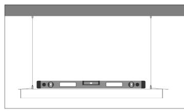
5. Adjust fixture until it is level and at desired height. Depress top of Cable Gripper to lower fixture. Keep fixture supported while lowering.
