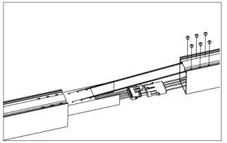
10. For custom runs, there may be multiple parts needed to be connected together as shown. Connect the wires quick connector together, then insert one of the rail with the other rail that has metal connector attached, then tighten with 6 screws. Repeat this step as necessary. Entire fixture need to be completely assembled before mounted on ceiling.
