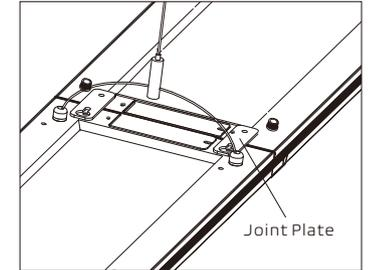
① Joint two luminaires together by mounting the Joint plate on the both sides as shown.
