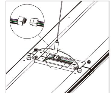
② Remove the existing covers, then connect the quick connectors properly.
