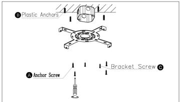
2. Install the mounting bracket to the J-box using screwdriver
