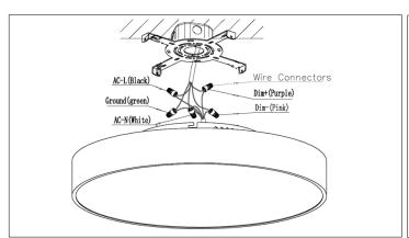
3. Make the wiring connection, and tuck the wires inside the J-box. Ensure Power is OFF prior to connecting wiring. CAUTION: Do not pinch wire connections.
