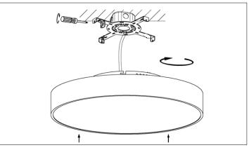
4. Push the canopy up towards the bracket, and rotate clockwise to secure. Tighten the 4 screws on the bracket to secure canopy.
