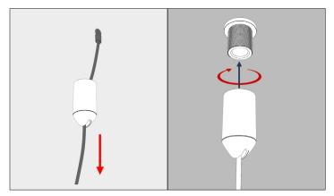
3. Route Suspension Cable through Suspension Bullet. Ball end should sit in Suspension Bullet. Screw Suspension Bullet to Ceiling Fitting.
