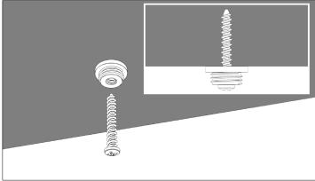
2. Canopy Fittings may be installed directly into framing with appropriate hardware.
