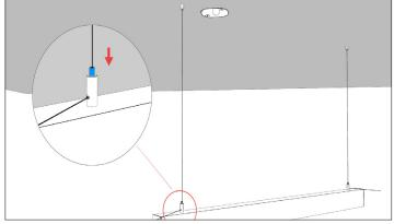
4. Raise fixture to Suspension Cables, and attach fixture by inserting Suspension Cable through Cable Grippers. Keep an extra 6 inches of cable for adjustments.
