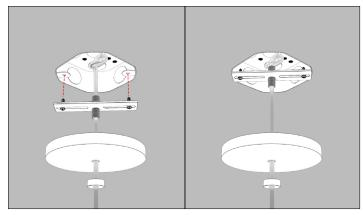
8. Mount Canopy Bracket to J-Box using provided screws. CAUTION: Do not pinch wire connections.
