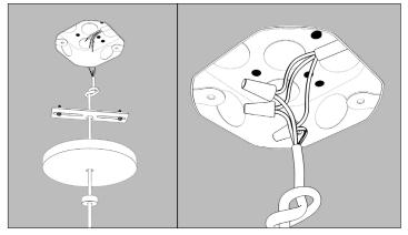
7. Bring wiring and canopy assembly to J-box. Refer to final/record drawing to make wiring connections. Ensure Power is OFF prior to connecting wiring.
